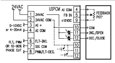
The UIPCM-AC uses two logic Triacs to switch the 24VAC outputs. The UIPCM can be configured with an optional feedback input for open or closed loop control.
